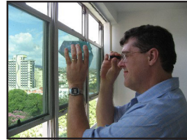
David Dow checking out dichroism with a “dichroscope” on large slice of aquamarine crystal. 7/2/2007, Photo by Tony Kampf
